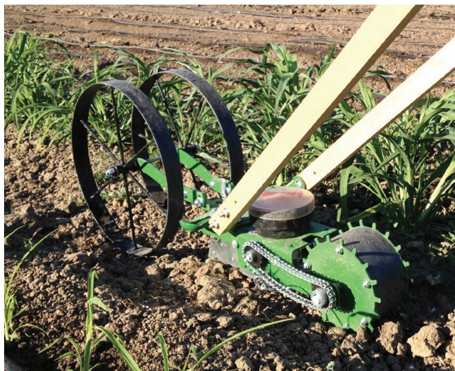
From top to bottom: At top: Farm School Director Antonia Partridge and a crew of visiting AmeriCorps volunteers celebrate the Planet Junior seeder. Middle: The seeder in action. Bottom: A close-up of the Planet Junior seeder, a hand-powered piece of equipment with a basic design perfected over a century ago.
