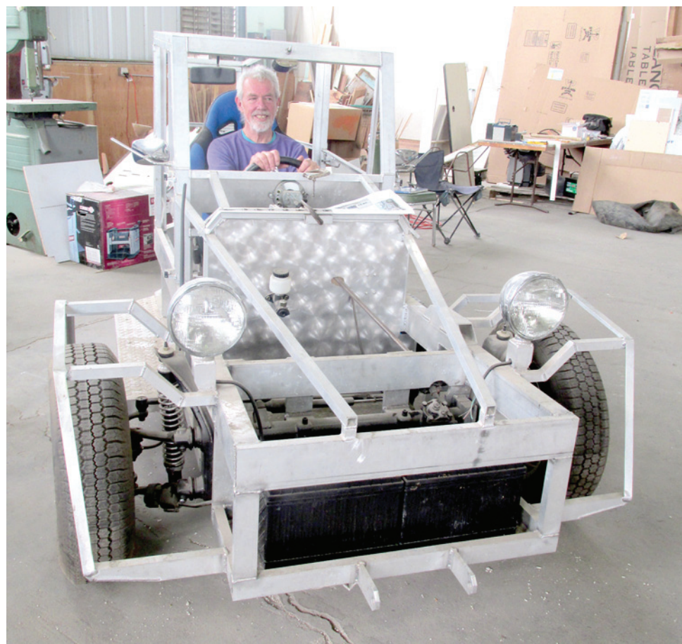
Above: Michael Hackleman in the "Silver Hawk" chassis he is turning into an electric vehicle. The steel chassis was built by Ron of Mendocino Tool and Machine and welded by Keith of K-Arrow Welding.
